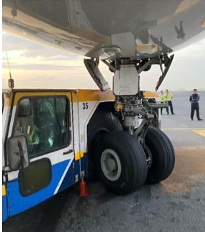
Photo 1: NLG impacted with the Left Hand Side of the Tractor
