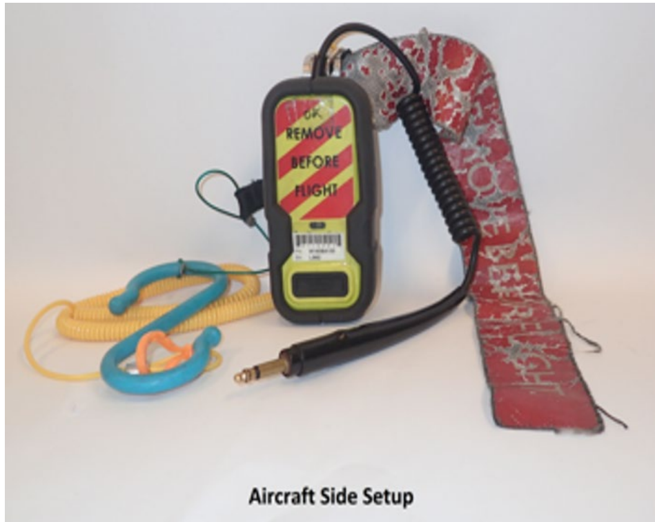
Photo 3: Wireless Headset Setup for Aircraft Side
