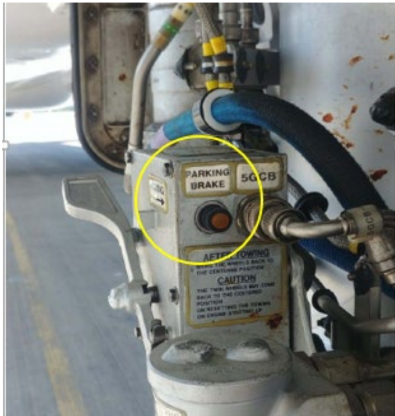
Photo 4: Parking Brake Light on the NLG
